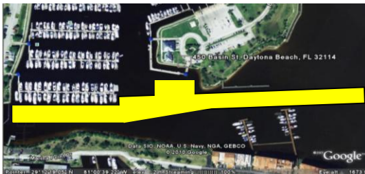
South Basin Entrance Channel Dredge Area
